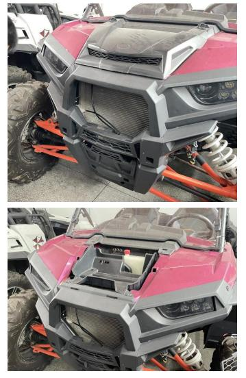
3. Install the new mesh grill, first pull the wiring harness of the mesh grill spotlight through the gap of the vehicle to the battery wiring, and connect the positive and negative wiring harness of the spotlight to the battery, and then install the new mesh grill. As the picture shows:
