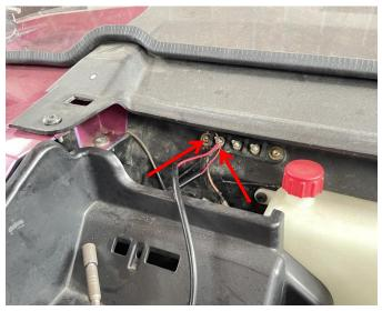
4. Remove the double-sided adhesive anti-mucous membrane on the surface of the spotlight drive box, and stick the drive box to the spare place of the original vehicle, and then start the vehicle to check whether the
