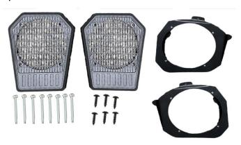
1. First distinguish the left and right sides of the iron brackets, then use M6\*16 self-tapping screws to fix it on the roof of the original vehicle (the roof has reserved fixed columns), and finally use M5\*30 screws to install the speaker and speaker pod on the iron bracket (the other side is installed in the same way). As the picture shows:
