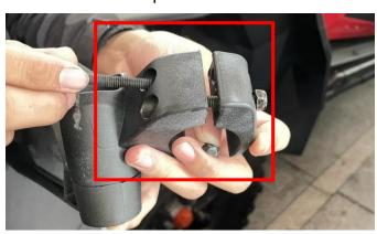
2. Clamp the side mirror on the A-pillar frame of the original vehicle, adjust it to the appropriate height, and tighten the screws on the mounting bracket. Install the other side in the same way. As the picture shows:
