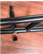
3. Install the side bar to the three mounting holes at the lower end of the vehicle frame.
