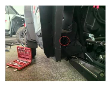
4. Tighten the 6 mounting screws, and then tighten the 12 connecting M8 screws.
