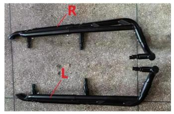
2. Install the casting on the side bar with six M8\*55 hex screws and six M8 flat washers, do not tighten the screws.
