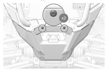
2. Remove two lower winch cover fasteners.
