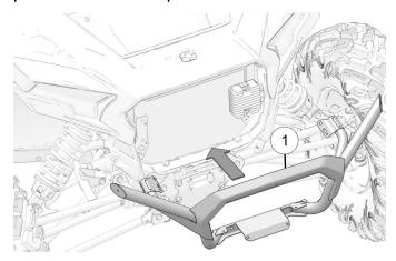
2. Loosely install front of bumper with two nuts (2).
