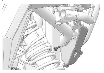
2. Remove one push-pin rivet from each side of front fascia.
