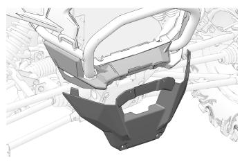
2. Install winch cover with two retained fasteners. Torque fasteners to specification.
