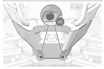
3. Install winch cover with two retained fasteners. Torque fasteners to specification.
