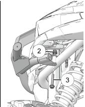
4. Torque two front nuts to specification.
