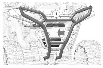
2. Put two bolts (2) through lower bumper mounts and through transmission bracket.
