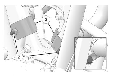
6. Hold weld plates in position and torque two bolts (2) to specification.
