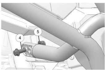
4. Put one bolt (4) through bumper and mount. Loosely install bolt with one nut (5).
