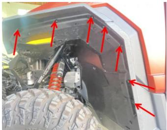
3. Prepare an 8mm drill bit, drill holes in the original vehicle according to the fixed holes on the fender flares, and then fix it with regular snap fasteners (the position shown in the second picture needs to be fixed with a big-head snap fastener). As the picture shows:
