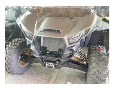
3. First, disconnect the wire harness of the central grille light and connect the disconnected end of the wire harness to the original vehicle headlight daytime running light wire harness using a broken skin method (black wire to black wire, red wire to brown wire). The interface needs to be insulated and protected. Finally, pull the connected wire harness through the vehicle gap to the central grille and re connect it with the wire harness plug on the central grille. As shown in picture:
