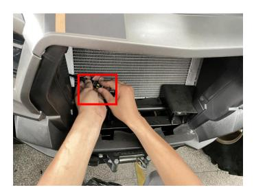
4. Finally, start the vehicle to test whether the grille lights are working properly. After confirming that they are correct, remove the double-sided adhesive film on the surface of the drive box, stick the drive box to the gap between the original vehicle, and then install the original vehicle hood. As shown in picture:
