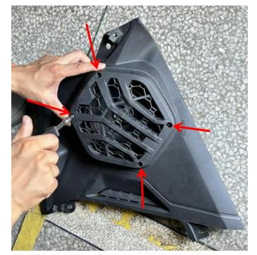
4. Remove the original hood, both sides of the instrument panel and the A-pillar panel, and transfer the steel clips on the panel to the speaker bracket.
