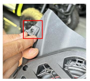
5. First distinguish between the left and right speaker brackets and install them on both sides of the vehicle's dashboard, using the original screws to secure them.
