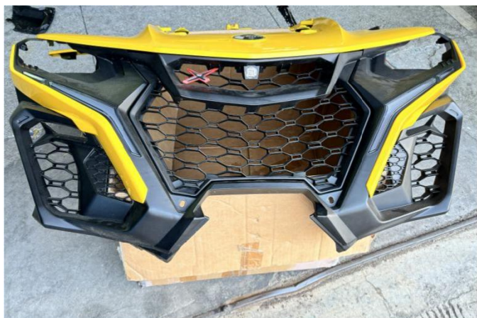
6. Reinstall the front fascia with the replacement daytime running lights back into the original vehicle and connect the wiring harness plug-in for the daytime running lights.
