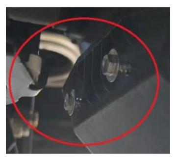
5. Fix the rear guard to the frame with 2 clamps, M6\*20 screws and M6 nuts, and the center position is fixed with M10\*30 self-tapping flange screws.
