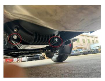
4. Secure the front guard under the frame with 4 self-tapping screws.
