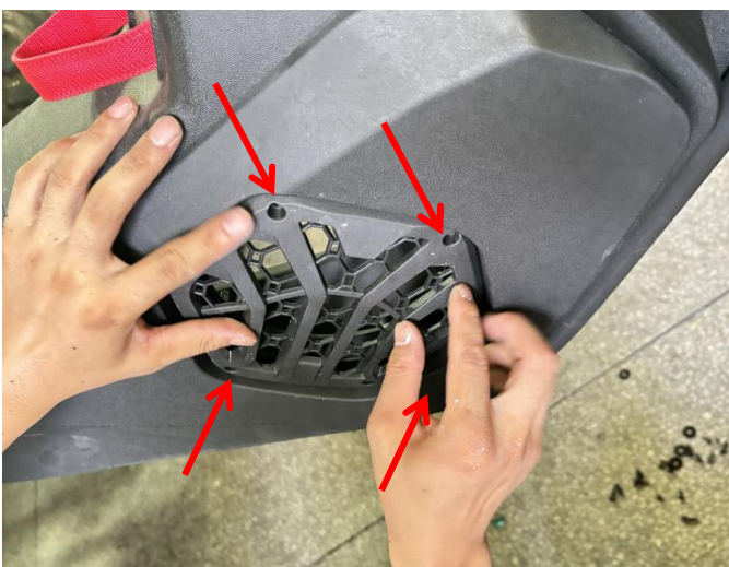
6. After installing the speaker, you can use M4 *16 self-tapping screws to fix the sound decorative frame on the speaker bracket, and then finally install the vehicle's original exterior door panels back to the original position can be (the other side of the speaker bracket according to the same way as above to install).
