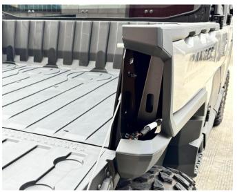
3. Attach the steel clamp of the new taillight to the back housing, then connect its plug-in to the vehicle, and then install the taillight.
