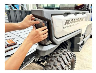
4. Finally, use the matching screws and the original screws to fix it. (The other side can be installed in the same way.)
