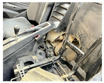
4. Connect the bypass with the seat belt buckle alarm plug-in of the vehicle. Then reinstall the decorative shell with buckles and seats. (Same ways to install the other side.) As the picture shows:
