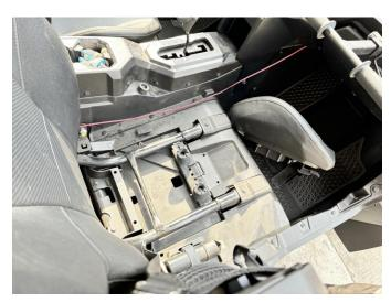
3. Remove gear lever decorative shell and its fastening buckle.
