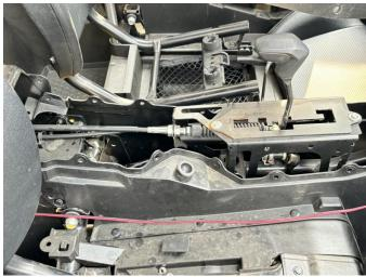
4. Connect the bypass with the seat belt buckle alarm plug-in of the vehicle. Then reinstall the decorative shell with buckles and seats. As the picture shows:
