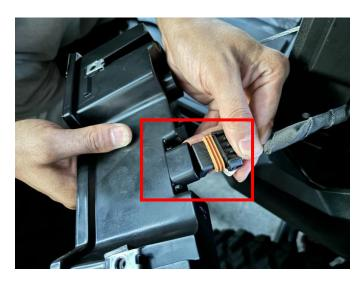
3. Start the vehicle, test whether the taillight is working properly, and then install the taillight after confirming it, and use M5\*30 screws to fix it. (The other side of the taillight is installed in the same way as above). As shown in the picture:
