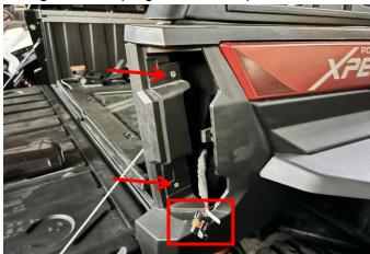
2. Install the steel clips in the kit on the rear shell of the new taillight, and then connect the wiring harness plug-ins of the original vehicle. As the picture shows:
