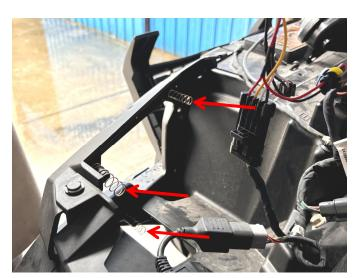
2. Distinguish the left and right sides of the new headlights in advance, connect the plug-ins of the headlights with the vehicle wiring harness, and then install the new headlights on the vehicle, and use the original screws of the vehicle to fix. As the picture shows:
