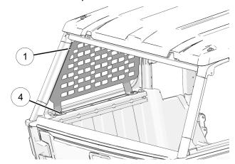
3. Install upper mounting hardware. Use screw (5) and nut (6) in hole closest to front of vehicle. Use screw(5), nut(6), and spacer(3) in hole closest to rear of vehicle. Position spacer between MOLLE panel and enclosure, as shown. Torque screws to specification.
