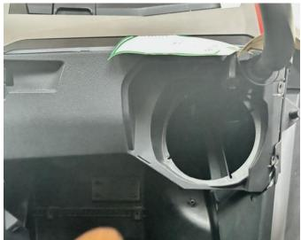
3. Install the speaker pod on the original vehicle, fix with 6.3\*19 and 4\*10 self-tapping screws, and finally install the speaker decoration net of the original vehicle back to the original position (the other side of the speaker pod can be installed in the same way). As the picture shows:
