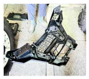
2. Remove the trim plates on both sides of the front fascia of the original vehicle, replace it with new trim plates, and fix them with the original screws (you can also use the screws in the product accessories package). As the picture shows:
