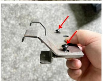
2. Fix the No. 3 and No. 4 mounting brackets (fixed in the direction of the brackets shown in the picture) on the speaker pod by using M6\*12 hex socket screws (Don't tighten the screws too tightly). As the picture shows:
