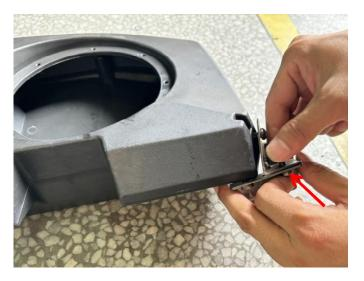
3.Attach the installed pod on the rear beam bar of the roof of the original vehicle, and after determining the position, fix the screws. As the picture shows:
