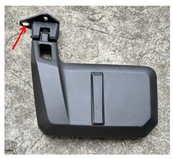
2. Place the bracket with nuts welded onto the inner wall of the A-pillar of the original vehicle, and ensure that the nuts on the bracket are aligned with the screw holes on the surface of the A-pillar (to facilitate the installation of the rearview mirror). As shown in picture:
