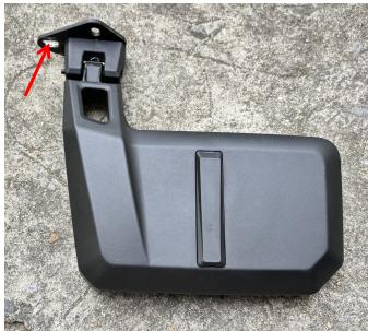
2. Remove the door liner plate is 2 nylon buckle, and lift the corner of the liner, and then prepare 6MM drill bit, according to the original holes on the vehicle for drilling. As shown in picture:
