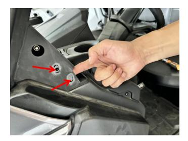
3. Use M6 \* 20 screws to secure the rearview mirror to the original A-pillar of the vehicle (the other side of the rearview mirror can be installed using the above method). As shown in picture:
