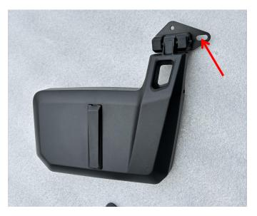
2. Remove the door lock on the A-pillar of the original vehicle, and then reinstall the installation bracket of the rearview mirror and the door lock back to their original positions (use the original vehicle screws to fix them first, and do not tighten them. The screw holes on the inner bracket need to be consistent with the screw holes on the surface for the installation of the rearview mirror). As shown in picture:
