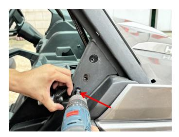
3. Use M6 \* 25 screws to secure the rearview mirror to the A-pillar and tighten all screws. (Install the other side according to the above method). As shown in picture:
