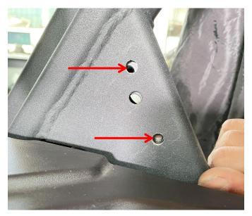
3. After completing step 2, the installation plate can be fixed to the original A-pillar with screws.As shown in picture:
