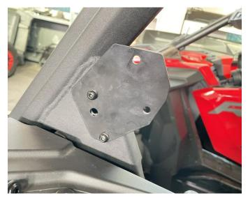
4. Fix the ball head bracket of the side mirror on the rear shell with self tapping screws (the
