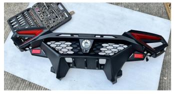
5. Reinstall the taillight bracket back into the vehicle as disassembled and reconnect the taillight as well as the wiring harness plug-in for the reverse camera.
