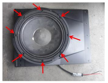
4. Use hex socket screws to fix the supporting iron bracket on the speaker bracket.
