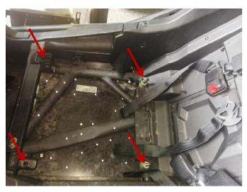
6. Install the speaker bracket under the seat (the iron bracket on the speaker bracket needs to be overlapped and aligned with the iron bracket fixing the pulley bar for subsequent fixing), then re-install the seat pulley bar, use the original screws of the vehicle for fixing, and finally install the seat back. (The other side of the speaker bracket is installed in the same way as above)
