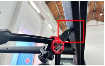
4. Use a special tool to rivet the rivet nuts from the kit into the pre-drilled holes in the top crossbar of the vehicle.
