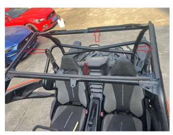
4. Install four M6 U-shaped clips on the top four corners of the frame, as shown in the figure:
