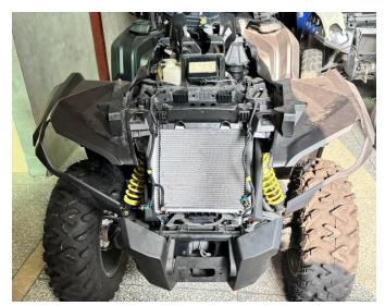
4. Remove the headlights from the old front fascia and reinstall them on the new front fascia. After the headlights are assembled, the new front fascia can be installed on the vehicle and fixed with the original screws (Install and fix in the original disassembly way). As shown in the figures:
