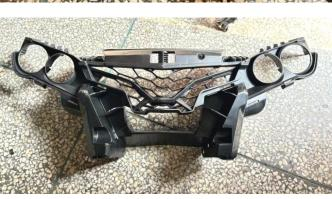
3. Unscrew the fixing screws of the dash protective cover and lift it. Then remove the front electrical box cover, the original front fascia, and the tow rope winch. As the pictures show:
