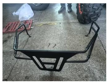
3. Remove the original three screws of the rear frame as shown in the picture, and the removed screw in the middle need to be reserved for use.
