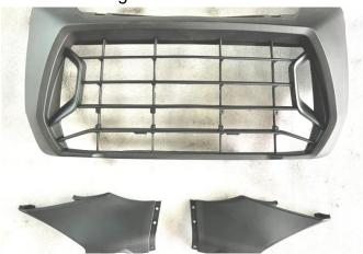
3. Assemble the separate front fascia as a whole, using M5\*16 screws with flat washers and nuts.
