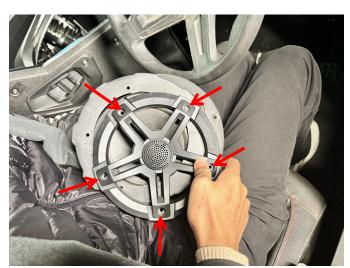
2. Find a suitable position on the roof to place the speaker pod, prepare a 6MM drill bit, drill holes in the screw holes of the pod, and fix the pod by using M6 screws, waterproof sponge pads, and nuts. As the picture shows:
