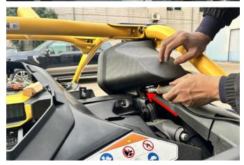
5. The self-provided audio speakers will be installed and fixed in the bracket, connect the wiring harness, you can use the decorative frame M4 \* 16 self-tapping screws fixed in the speaker bracket, and then finally back to the previously disassembled A-pillar base as well as the decorative plate can be installed. The other side of the speaker bracket is installed in the same way as above.
