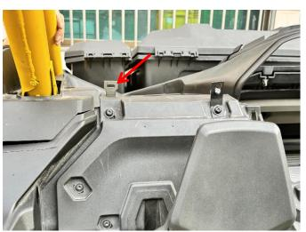
4. Remove the vehicle's rear A-pillar exterior decorative plate, loosen the screws on the A-pillar base plate (the base plate does not need to be removed, in order to follow up the screws), after which the speaker bracket is stuck on a matching steel card and the audio bracket is mounted to the vehicle, using M6\*20 screws for fixation.
