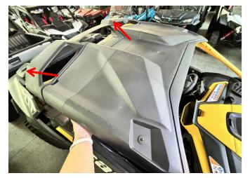
5. Finally, use nylon straps to pass through the roof mounting holes (both front and rear need to be secured with straps) and wrap around the crossbar for reinforcement.
