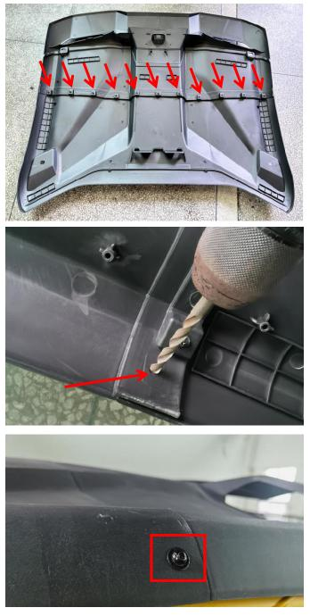
4. The assembled roof will be mounted on the vehicle, the front end of the roof using hexagonal M6 \* 25 screws and nuts for fixing (screws need to be set on the matching sponge gaskets and flat pads before use), the rear end of the roof need to use the special iron pressure plate and hexagonal M8 \* 25 screws and flat pads for fixing the nuts.
