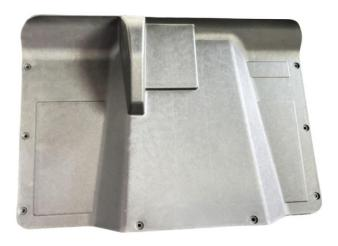
1. First remove the original partition board of the vehicle, then replace the new partition board, and use the original screws of the vehicle to fix it. As the picture shows:
