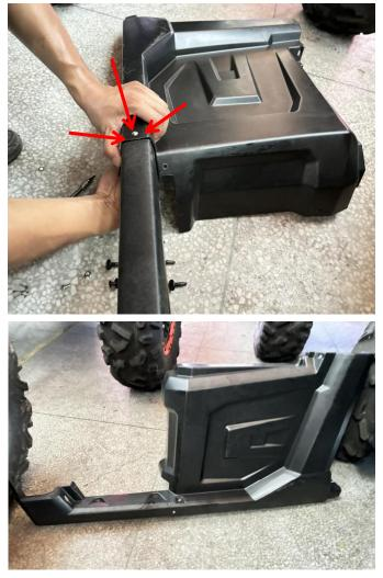
2. Remove the seat lower side guard plate of the original vehicle, replace and install the new guard plate in the original way, fix by the screws and the snap fasteners of the original vehicle (you can also use the matching screws in the accessory package), and finally reinforce by the self-tapping screws of the product. As the picture shows:
