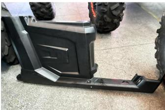
2. Remove the seat lower side guard plate of the original vehicle, replace and install the new guard plate in the original way, fix by the screws and the snap fasteners of the original vehicle (you can also use the matching screws in the accessory package), and finally reinforce by the self-tapping screws of the product. As the picture shows:
