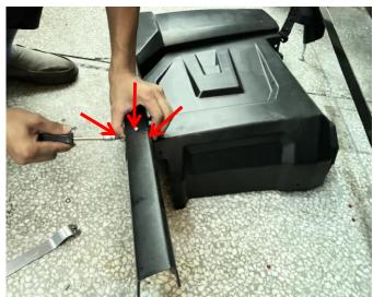
2. Remove the seat side guard plate of the original vehicle, replace and install the new guard plate in the original way, fix by the screws and the snap fasteners of the original vehicle (you can also use the matching screws in the accessory package), and finally reinforce by the self-tapping screws of the product. As the picture shows:
