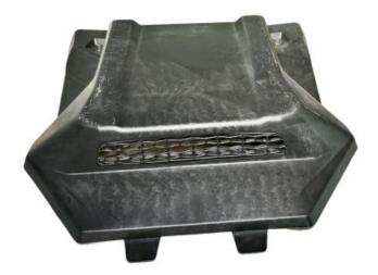
1. First remove the original hood scoop, and then replace it with the new hood, and fix it with the original screws. As the picture shows: **Note**: The two limit brackets need to be stuck into the notches of the original vehicle during installation.
