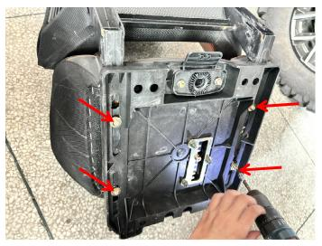
2. Remove the iron limit bracket from the original base and install it on the new base. Install the new base under the original seat and fix it with the original screws. As the picture shows:
