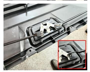
3. Insert the two limit pull rods into the fixing holes at the two ends of the door panel, install the door panel, secure it with the original screws, and then reinstall the screws on the inner door panel. As the picture shows:
