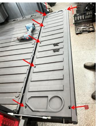
2. Remove the outer door panel, remove the limit rods and locks on both sides of the door panel, and move them to the new door panel. As the picture shows:
