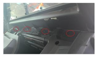
3、Connect the lower end of the rear windshield with the vehicle frame with two small straps
