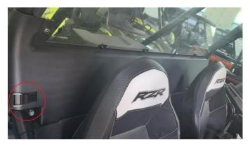
4. Connect the upper end of the rear windshield with the vehicle frame with six small straps, and the installation is completed.
