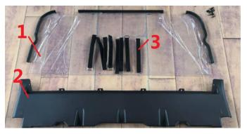
1. Install the rear windshield 1 on the plastic part 2 with 6pcs M6\*20 hexagon screws, 6pcs M6 Flat pads and 6pcs M6 lock nuts., as shown in the picture as above:
