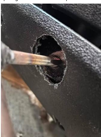
4. Install the nerf bar in the four mounting holes with four M10\*20 flange socket head cap screws and tighten the screws. As shown in picture:
