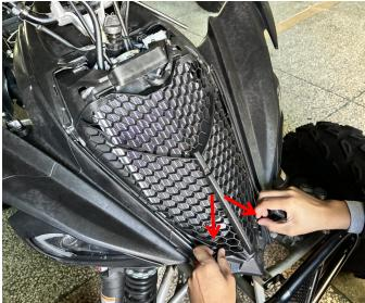
2. Finally, reinstall the decorative frame back into the original vehicle and secure it with the original vehicle screws. As shown in picture:
