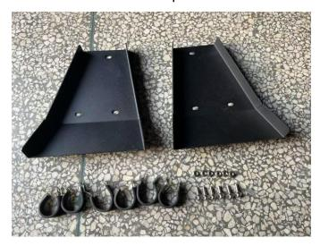
1. Secure the A-arm guards to the bottom of the front frame using 6 M6\*20 hex screws, 6 M6 flat washers, and 6 clamps. As shown in picture:
