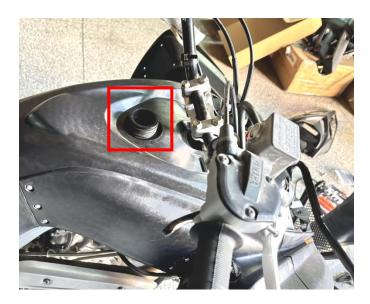
6. Remove the original vehicle front fender and fuel tank trim panel. As shown in picture:
