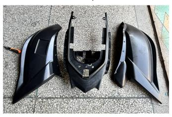
1. First, use the matching screws and nuts to assemble the rear fender into a whole. As shown in picture:
