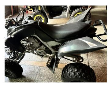
3. Install the newly assembled rear fender Newly and secure it with the original vehicle screws. Finally, fix the original vehicle insert and seat cushion. As shown in picture:
